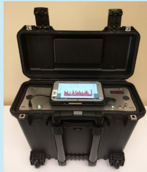
Figure 1. Field-deployable Multiplicity Counter for Thermal and Fast Neutrons [S81].
