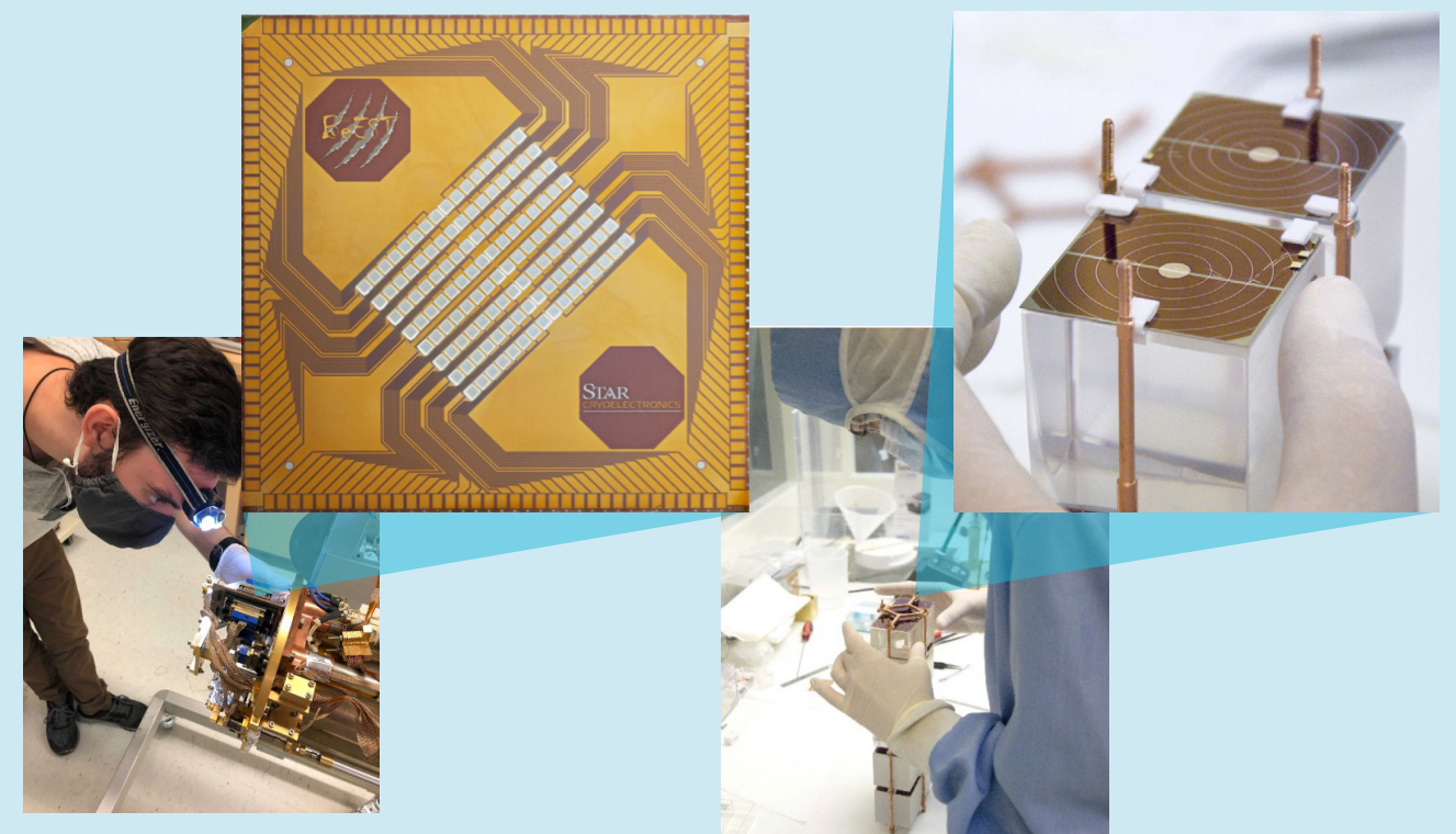
Figure 1. (left) A microscope image of a 128-pixel aluminum-based superconducting tunnel junction array prototype for Phase IV of the BeEST experiment. This type of array is implanted with large doses of radioactive beryllium-7 and operated at near absolute-zero temperatures to search for exotic new physics [S49-50]. (right) A CUPID scientist assembling cryogenic sensors based on scintillating crystals for quantum-enabled light detection [S51-52].
