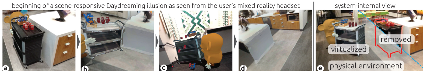
Figure 1: We present Scene Responsiveness , the visual illusion that virtual actions affect the physical scene. (a) Wearing a video-passthrough Mixed Reality (MR) headset, a user sees an authentic video view of their physical environment, captured with the externally-facing headset cameras. A virtual monkey character is situated and coherently occluded in the otherwise unmodified physical space, grabbing the PHYSICAL cart. (b) As the monkey starts dragging the cart, the object toggles its reality state to VIRTUALIZED just-in-time. Just-in-time virtualization is coherence-preserving , so the cart still throws its shadow onto the physical scene and the now seemingly empty surface. (c) To the user, it appears as if the monkey drags the physical cart and throws it down the staircase. Virtual shadows and collisions render coherently. (d) It appears as if the physical cart is gone. (e) Of course, what the user sees is just an illusion. The physical object did not move but was just masked from the user's view, blending seamlessly with the video passthrough. Everything seen in the debug capture, incl. the red object guardian outline and the revelation lens in the top-right corner is part of the system debug view. The figure gives an authentic impression of the visual fidelity in the headset. However, please watch the accompanying video for a full impression of the visual experience.
